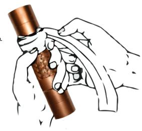
3. Direct all heat away from the base of fitting and hose/braid. Avoid any open flame contact to this area as well.
