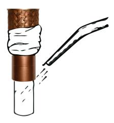
4. Use silver solder to connect the assembly to the system.
