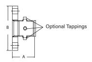
FG - Flange and Groove RFG - Reducing Flange and Groove
