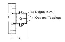
FW - Flange and Weld RFW - Reducing Flange and Weld
