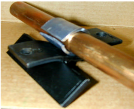
3. Mold shim to pipe on upper half, lay shim on inside of spider clamp
