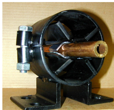
6. Complete unit shown for copper pipe and lead insert installed.
