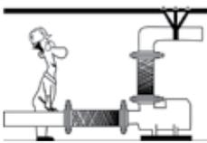
**DO USE HANGERS AND PIPE GUIDES** on all adjacent piping. Install hangers and guides before installing hose, to be certain weight of pipe is on the hangers and guides.
