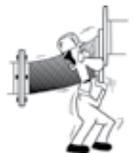
**DON'T LET WELDING SPARKS HIT THE BRAID;** they may burn some of the braid strands. Protect the metal hose braid with a non-flammable cloth or place another type of non-flammable protective material in front of it when piping must be welded very close nearby.
