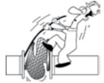
**DON'T STRETCH** the connector to fit a gap longer than its factory-furnished length. Stretching the connector places excessive residual stresses on braid and fittings, thus ultimately resulting in rupture.
