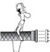
**DO LINE UP BOLT HOLES.** Make sure all bolt holes are perfectly lined up before welding pipe flange into place. It is best practice to use a floating flange on one of the connector's ends to allow for bolt hole alignment in the field.
